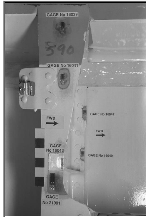
Figure 1. Strain gauges installed on the aft fuselage in the vicinity of the vertical tail.
